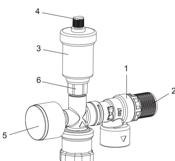
The pressure relief valve (1) can be activated manually by turning the knob (2). By turning as indicated by the arrow the valve is opened and will automatically close again. The function of the valve can be tested and the area of the valve seat can be flushed free of debris in this manner.
