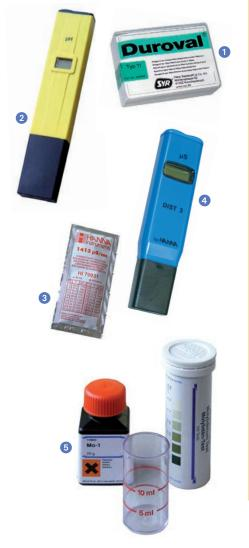
The pH of the filling water and conductivity are the relevant values for the correct heating water quality. To measure the hardness of the filling water, SYR offers two direct, on-site measurement methods.
