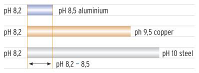
If, for example, the installation is fitted with the three materials aluminium, copper and steel, the pH of the heating water should be between 8.2 and 8.5 - this is where the protected range of the three materials overlaps, so that corrosion cannot occur.
