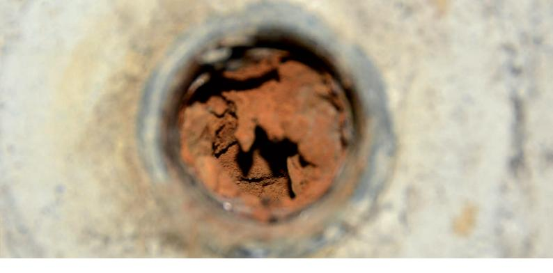
which serve as a natural protection against corrosion. Aluminium plays a special role here. The surface layers on aluminium parts (heat exchangers, radiators) can be damaged as from a pH of 8.5.
