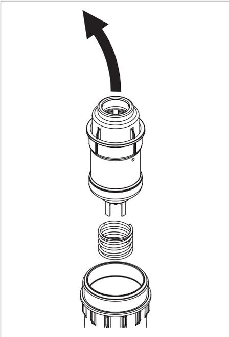
First remove the cover and then take the pressure reducer cartridge out of the sleeve.
