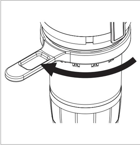
Remove the pressure reducer cartridge together with the suction casing and the suction pot by pulling out upwards. The spring remains in the filter cap.
