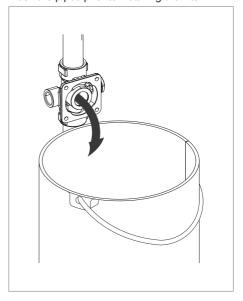
Install the heating system filter preferentially in the return pipe. However, it is also possible to mount in the supply line of the heating installation.
