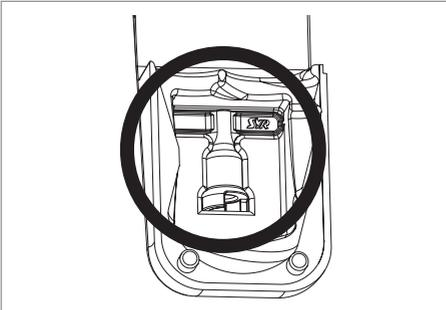
Remove the clamp from the control unit so that it can be lifted and taken off.
