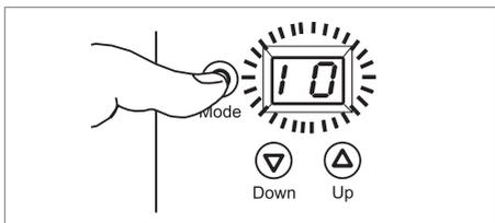
The system is open when the message 10 flashes in the display. Afterwards, it goes into the normal operation mode.
