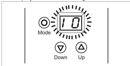
When pressing the Ⓞ - key, the system goes into the open position.
