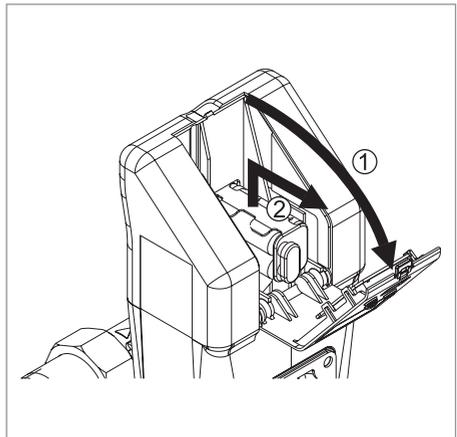
Insert the battery block or exchange it (4 x LR 06) and put it back into place in the battery compartment.
