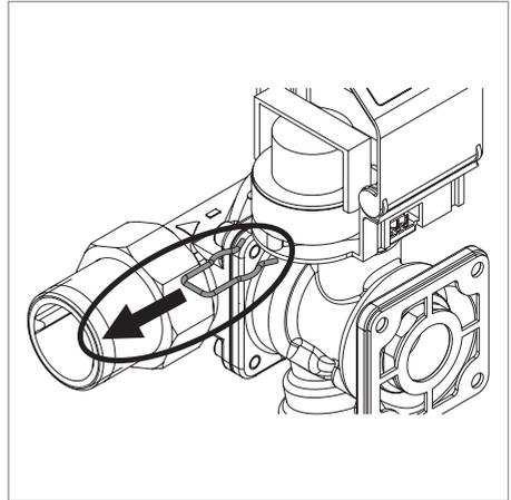
Put the key in the required position and turn it in the direction of the arrow until the water flows again.
