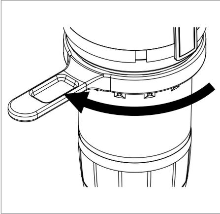
Remove the pressure reducer cartridge together with the suction casing and the suction pot by pulling out upwards. The spring remains in the filter cap.
