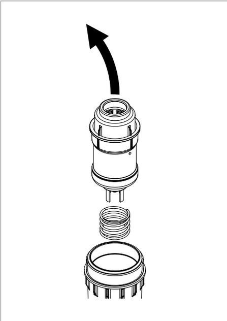
First remove the cover and then take the pressure reducer cartridge out of the sleeve.
