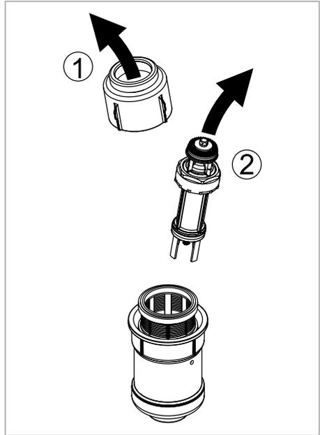
Clean the cartridge's diaphragm with cold and clear water.
