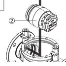
check valve (2) by means of the tool 6600.65.904.
