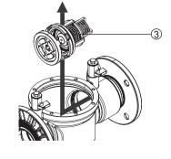
Turn the tool by 180° Disassemble the secondary check valve (3) by means of
