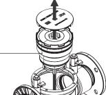
Remove the control unit (4) by means of the second tool
