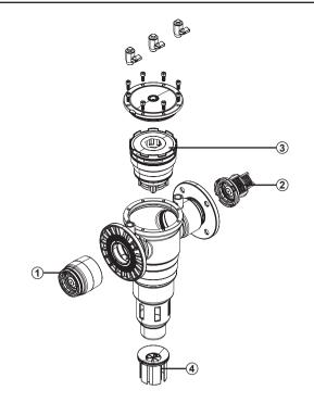
Check valve cartridge inlet
